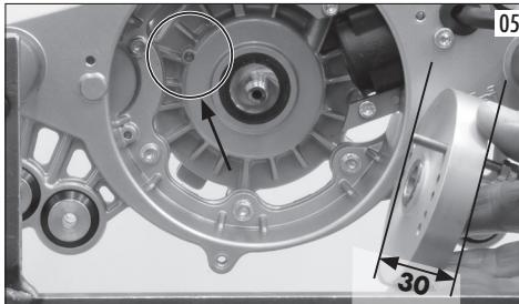
Screw the flywheel nut without locking it so that the crankshaft can rotate in the flywheel. Screw the comparator support into the spark plug hose, house the comparator and move the piston to the top dead centre. Now reset the comparator and rotate the crankshaft anti-clockwise of 1,2 mm towards the flywheel sense (see arrow in photo 6).
