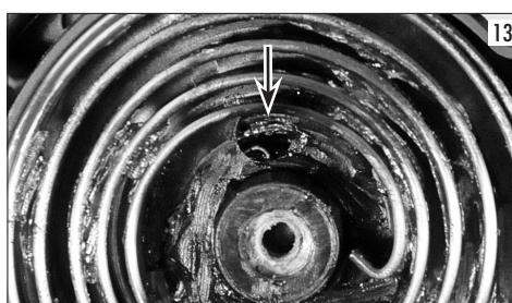
Now go on by charging the return spring: take the head of the rope leaving 10-20 cm coming out the hole with "u" shape on the wheel side. Turn the wheel three times in counter clock-wise sense till it stops in front of the exit hole on the aluminium case. Keeping the plastic wheel stopped, pass the rope through the case hole. Insert the handle and the washer and tie a single knot as shown in photo 14.
