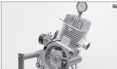
Once achieved the value, keep the pulley or the crankshaft stopped using one hand and tight the flywheel nut using a key, without exceeding. Check that the advance timing is as indicated (1,2+/- 0,1), remove the m.5x30 screw and fit the coil. Before locking it with the 2 screws, place between coil and flywheel one 0,35 mm calibrated shim (photo 7). Now definitely tight the flywheel nut using a torque wrench at 40Nm (photo 8).
