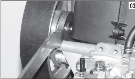
On the other side of the lever there is another bent side: place a weight of 6 kg on it. If you do not have the weight to place on it use a holder of 6 lit. and fill it till you reach the right weight.
