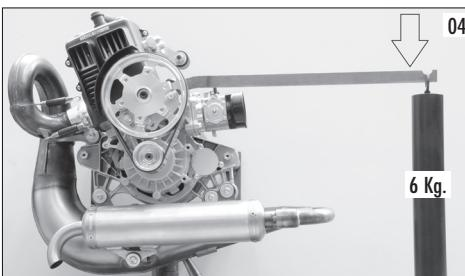
Now slightly push the lever with its weight downwards (as indicated by the arrow in photo 4), increasing of about the double the weight fitted. Then take the hand off and let the weight act on the lever by itself. Now tighten the M7 nuts again starting from the left one with 15Nm (1.5 Kgf.m) tightening. Remove the weight and the lever and fit the propeller.
